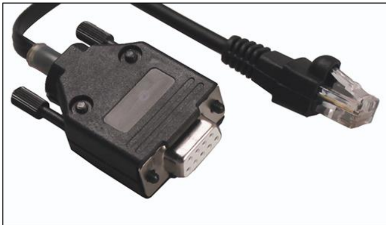
Figure 1: Left RS232 plug (D-Sub), right western plug
